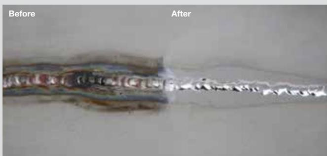
Electrochemical polishing is a process which removes parent material from the work piece and brightens the weld. This process will alter the surface and is mostly used to clean welds on mirror finished material. Electrochemical polishing is done on DC (Direct Current) mode available on the SURFOX MINI and SURFOX 204.
