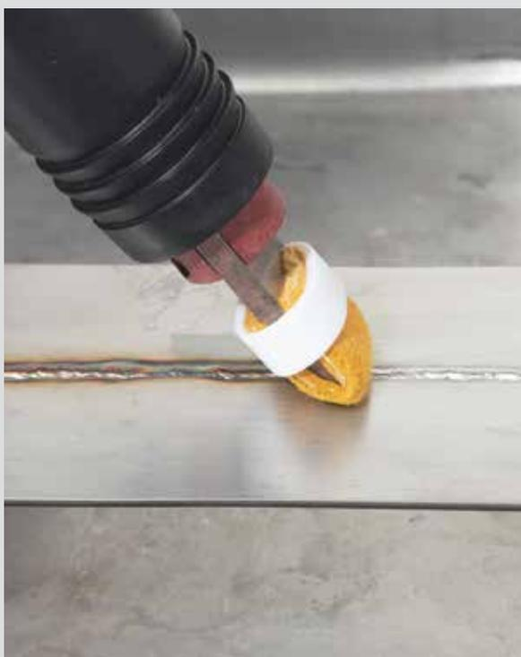
Passivation occurs when the chromium contained in the stainless steel comes in contact with the oxygen in the air. This chemical reaction forms a passive chromium oxide layer, which will protect the surface of stainless steel. To form a thick and uniform chromium oxide passive layer, the surface of the parent material must be perfectly clean and free of any contaminants.
